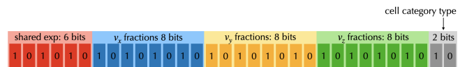
Fig. 6. The bit_struct for a 3D smoke simulation voxel. Three components of velocity ( v_x, v_y, v_z ) share one common exponent which is placed in the highest 6 bits. The fractions of velocity occupy 24 following bits. The cell_category is placed in the lowest 2 bits.
